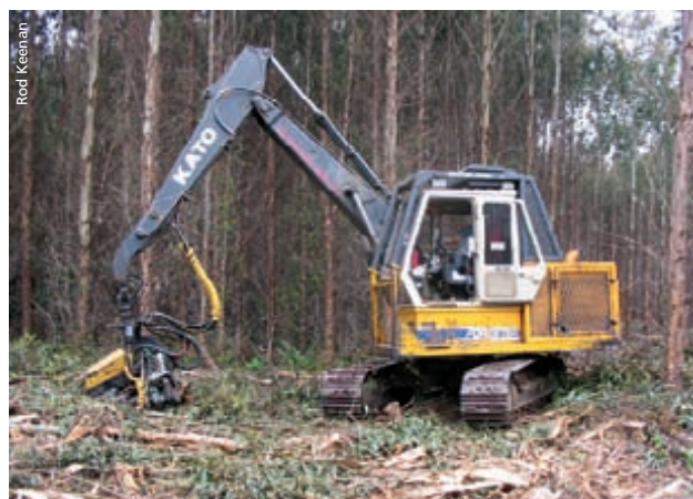
Depending on soil type and weather conditions, the choice of machinery, wheeled (above) or tracked (below) may determine the intensity of impact on soils during harvesting.
