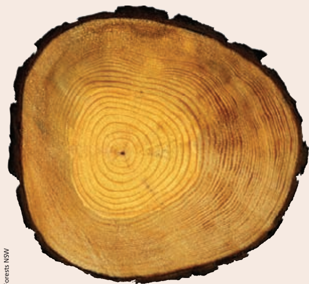
Cross-section of radiata pine ( Pinus radiata ). Annual growth sequesters carbon dioxide from the atmosphere; wider rings near the centre indicate faster growth and therefore more rapid uptake of carbon dioxide. During photosynthesis, about one tonne of carbon dioxide is captured from the atmosphere and combined with water taken up from the soil to produce about one cubic metre of wood. About 0.7 tonnes of oxygen is returned to the atmosphere.
