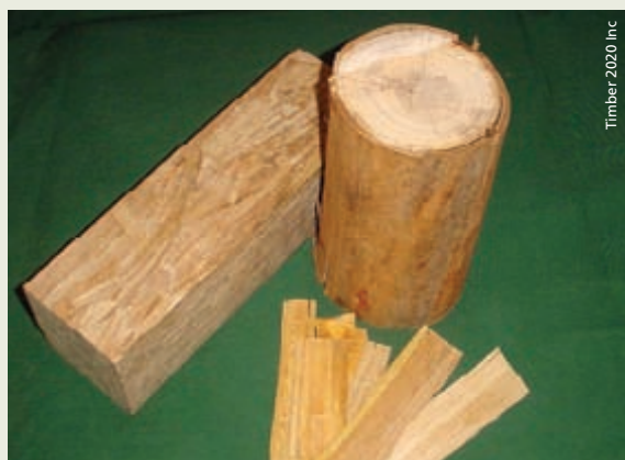
A plantation hardwood log is reduced to strands which are mixed with resin and compressed under heat and pressure to produce lumber.
